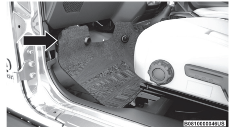
Front Carpet Pulled Away
