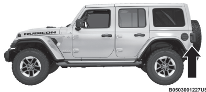
BSM Radar Location (Left Side Shown)
