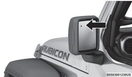
Warning Light Location
