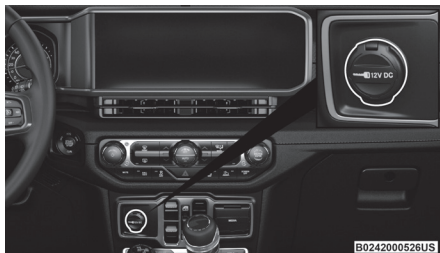
Front Power Outlet
