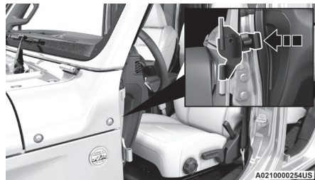
Push Bracket Onto A-pillar
